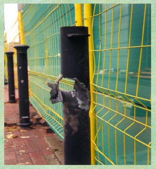
An example of bomb blast fragmentation damage
